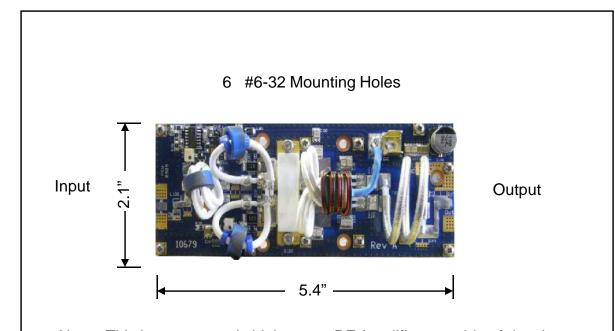
Note: This is an extremely high power RF Amplifier, capable of drawing more than 30A @ 43VDC. Use at least 12 ga. wire to supply DC power to this pallet. Although this is a very high efficiency amplifier, adequate cooling must be provided.
